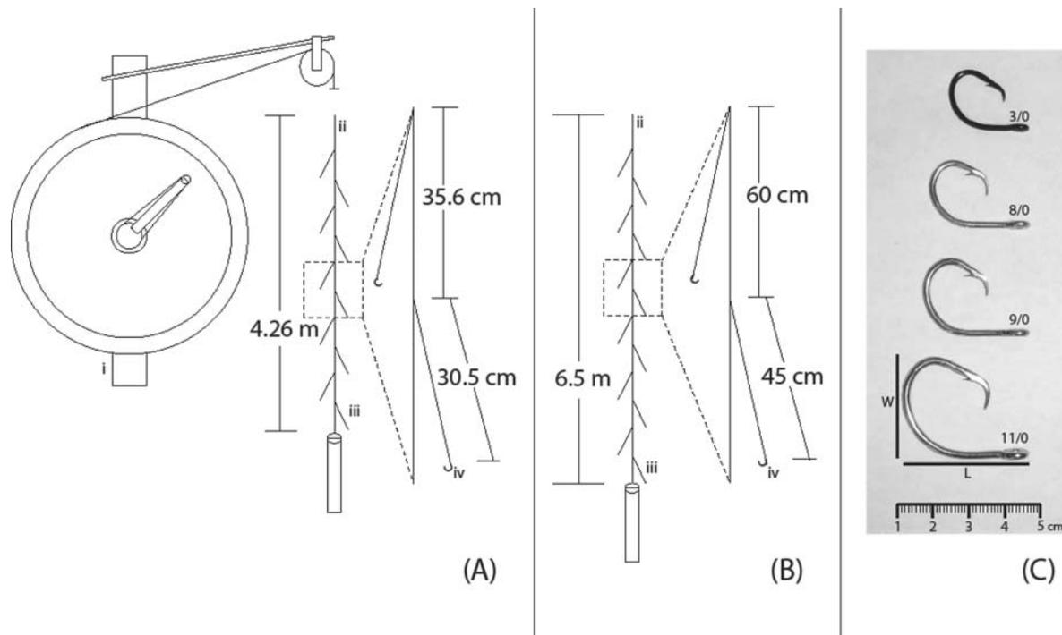
FIGURE 2. Gear configuration for vertical longlines used during (A) March–April 2010 and (B) May–November 2010; and (C) size range of hooks used in the current study (i = bandit reel; ii = backbone; iii = sash weight; and iv = gangion).
