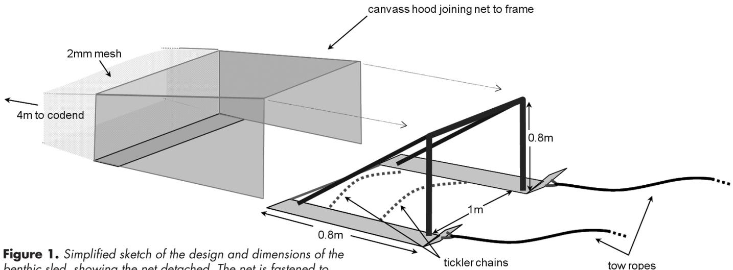
**Figure 1.** Simplified sketch of the design and dimensions of the benthic sled, showing the net detached. The net is fastened to the frame along the vertical and horizontal forward frame, along each skid and to the cross—bar at the rear of the two skids.
