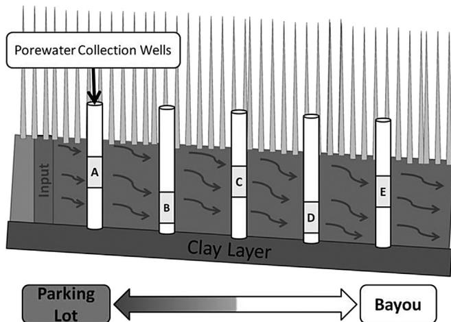
**Fig. 2.** Cross sectional view of one plot. The diffuser plate where the SGW was introduced is the input; the solution traveled down the plot (parking lot to bayou) as indicated by the black arrows. Wells were buried to the impermeable clay layer and screened at set distances below the sediment surface. The labeled region on each well represents the area that was screened (10–20 cm for A, C and E and 20–30 cm for B and D).
