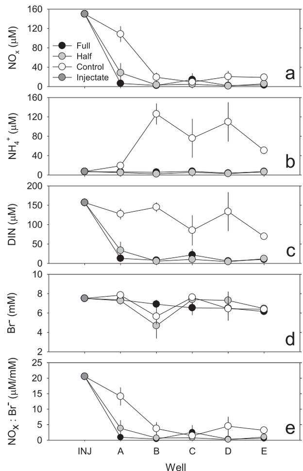
**Fig. 5.** Mean porewater chemical concentrations in the injectate (INJ) and each porewater collection well. Black circles represent the full density treatment, gray circles are the half density treatment, open circles are the control (non-vegetated) treatment, and the dark gray circle is the injectate concentration. Panel a is  $\text{NO}_x$ , b is  $\text{NH}_4^+$ , c is DIN, d is  $\text{Br}^-$  and e is the ratio  $\text{NO}_x:\text{Br}^-$ . Error bars indicate  $\pm 1\text{SE}$ .
