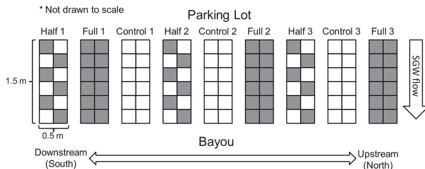
Fig. 1. Experimental layout schematic. Each shaded square represents one transplanted sod with dimensions of  $25 \text{ cm} \times 25 \text{ cm}$  and a depth of 30 cm. SGW flow direction went from the parking lot toward the bayou and this flow is depicted by the arrow on the right side of the figure.
