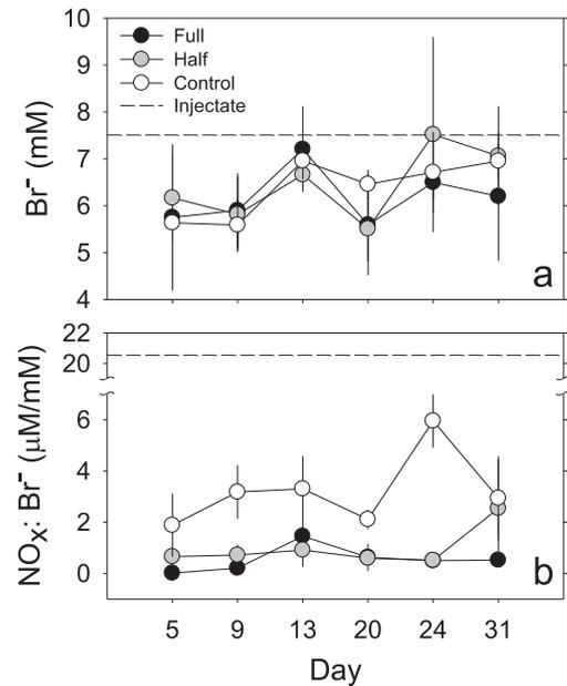
Fig. 3. Mean porewater chemical concentrations in well E through time. Black circles represent the full density treatment, gray circles are the half density treatment, open circles are the control (non-vegetated) treatment, and the dashed line is the injectate. Panel a is  $\text{Br}^-$ , and b is the ratio of  $\text{NO}_x:\text{Br}^-$ . The x-axis is not to scale. Error bars indicate  $\pm 1\text{S.E.}$
