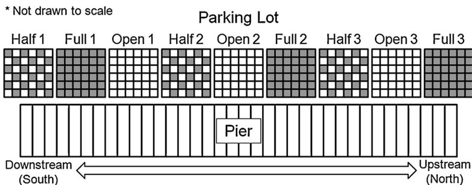
**Fig. 1.** Schematic of marsh construction layout with blocks 1, 2, and 3 proceeding from left (South) to right (North). Each block consist of a half density, full density and open treatment. Planted sods are indicated by shaded squares.
