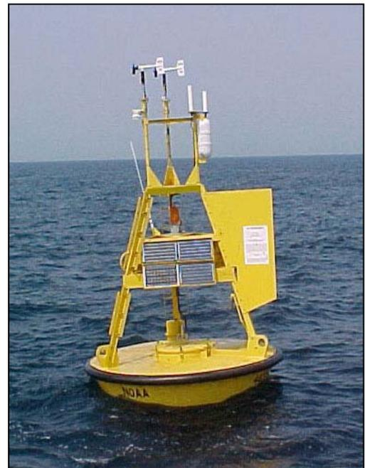
All buoys and many C-MAN stations located in offshore areas operate on marine batteries which are charged by solar cells. Data collection, averaging, and formatting for satellite transmissions are controlled by a payload computer system. On buoys, the payloads and batteries are located inside the hull; on C-MAN stations, they are located at the base of the tower.
